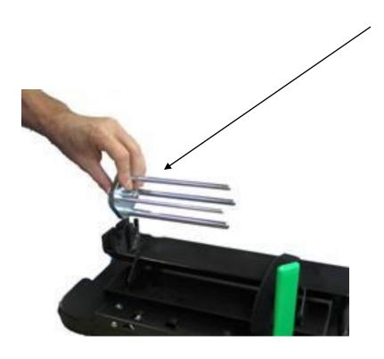
Remove the alternator mounting turret from the cradle.
